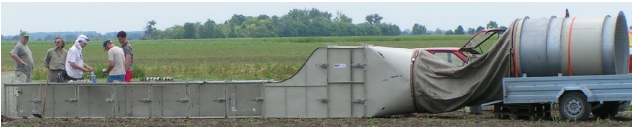
Fig. 4 The portable wind tunnel
